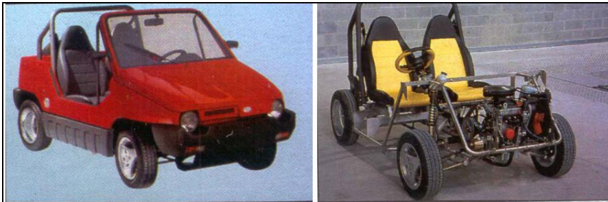
Fig. 7 Isigò, one of the first examples of stainless steel frame on a micro-car
