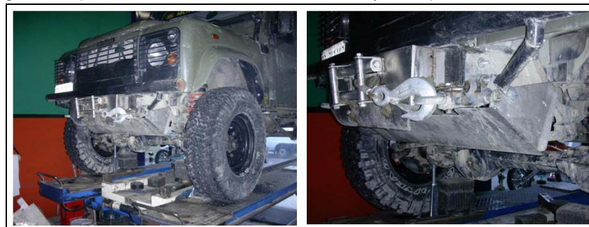
Fig. 3 The aspect of a stainless steel structure after three years exposure to road environment
