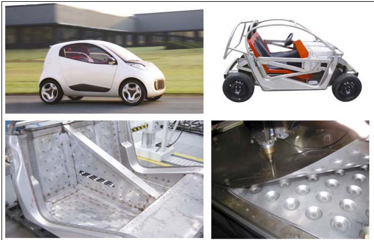
Fig. 10 The car prototype Nido with some details of the stainless steel structure
