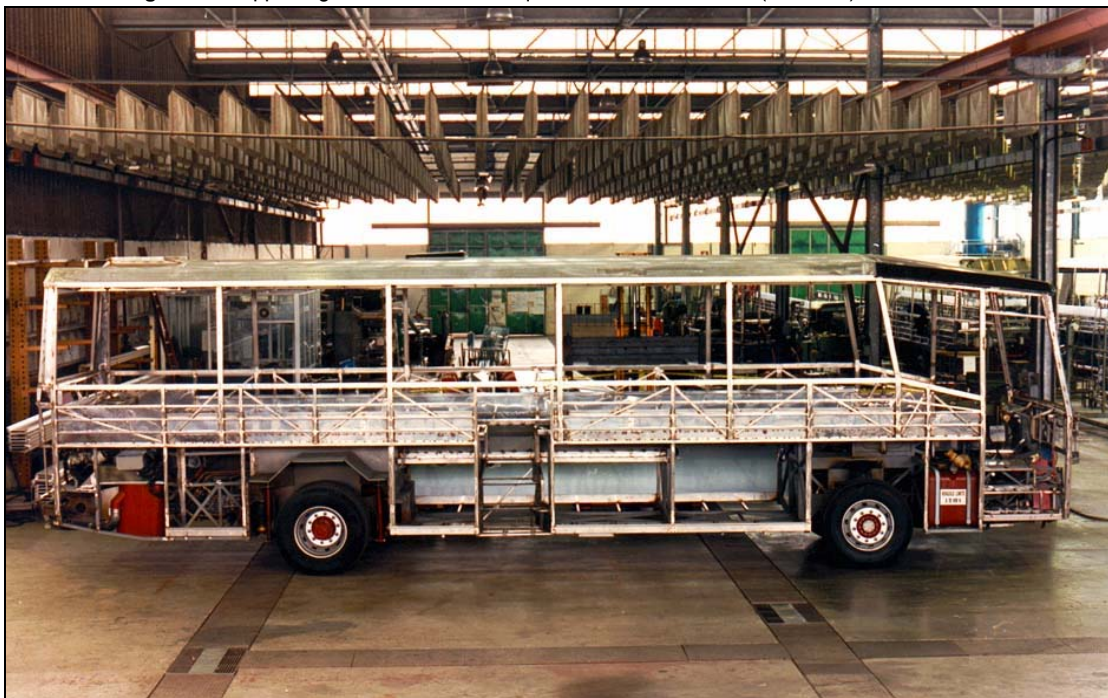
Fig. 6 Self-supporting bodies made with square section EN 1.4301 (AISI 304) stainless tube
