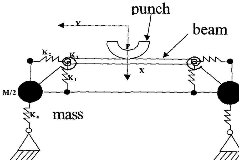
Fig. 4. Simplified model of beam and car body system for side impact simulation.
